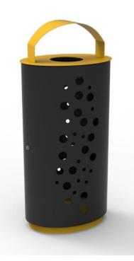
The elliptical-shaped bin is made of cold-rolled steel sheet, with a 3 mm top cover in a colour corresponding to the type of waste. The hinged front door is made of 1 mm steel sheet and is die-cut. The door is attached to the interior structure by a welded piano hinge. It is closed with a sliding lock mechanism with an 8 mm triangular cylinder.
