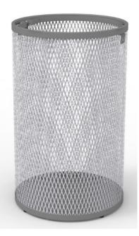
Large capacity waste bin, made of steel net, with upper ring made of 3 mm. steel plate, which tilts on a 3 mm. steel turning axis welded to the body, as well as a 3 mm. steel support welded at 180° to the axis.
