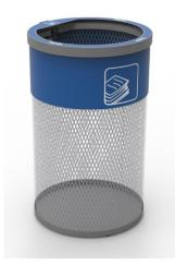
Large capacity waste bin, made of steel net, with upper bag holder ring made of 3 mm. steel plate, which tilts on a 3 mm. steel pivot shaft welded to the body, as well as a 3 mm. steel support welded at 180° to the shaft. Hinged head made of 1 mm thick stamped steel, labelled with high adherence vinyl according to the type of waste.
