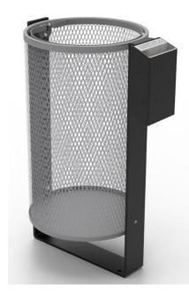
Large capacity waste bin, with structure made of extruded 6063 T4 aluminium alloy plate, 100 x 10 mm, shaped and finished in textured anthracite colour, and with 4 holes in the lower part that allow it to be anchored to the floor.
